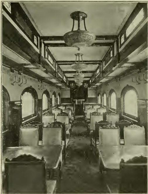
Alexalite Indirect Lighting Units.
